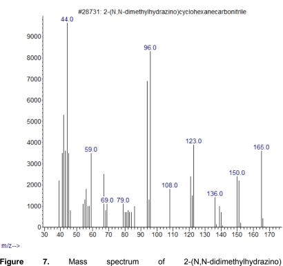
Figure 7. Mass spectrum of 2-(N,N-didimethylhydrazino) cyclohexanecarbonitrile.
